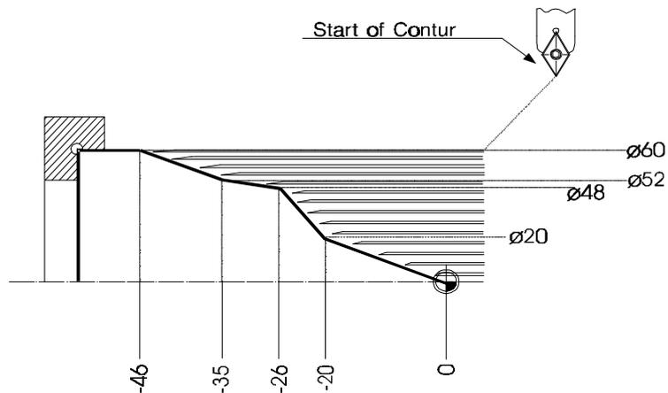
**Contur definition must start with bloc number N10 !** Allowed are G01, G02, G03!
