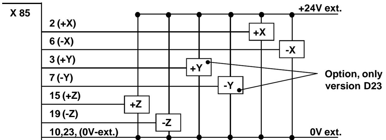
If the CNC should fail, no danger causing movement is allowed to result. Therefore, safety limit switches generating an emergency stop with power shut down, should be located after the normal limit switches.
